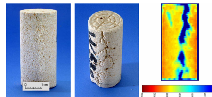
Figure 2: Core photos prior to and (left) and after (center) injecting a CO 2 rich solution and tomographic image (right).
