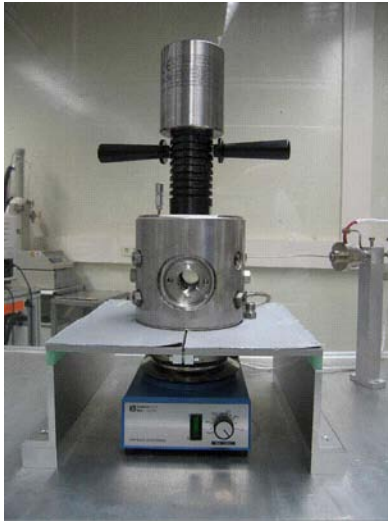
High p-T autoclave for measuring CO 2 -brine mixture properties up to 200°C and 50 MPa
