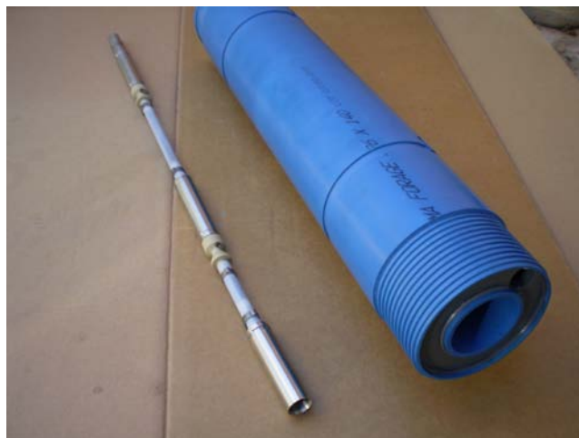
Figure 7. View of a double cask PVC section and the assembled electronic bus to be fitted between the inner and the outer shell.
